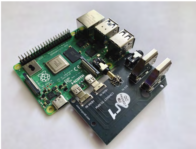
▲ The Argon One's clever expansion board brings all the connectors to the back and converts the HDMI ports to full-size
