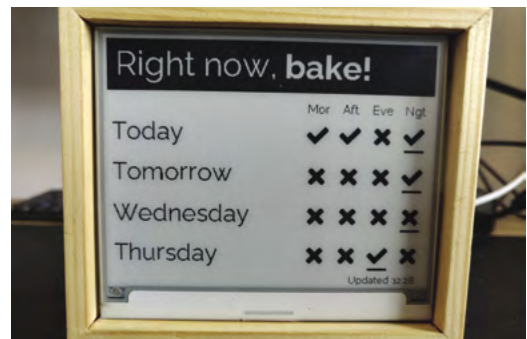
▲ Using his ShouldIBake project, Andrew schedules sourdough loaf baking when the maximum amount of energy to heat the oven comes from renewables
