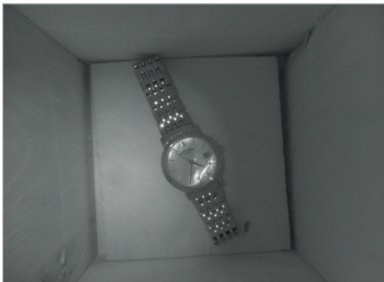
Fig 9 Make sure that the test object is raised up slightly and the text is in focus
