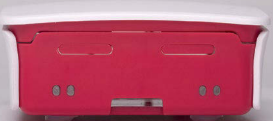
Above This fake case has two sets of light pipes Below The shoddy feet on this case are a clear sign of a fake
